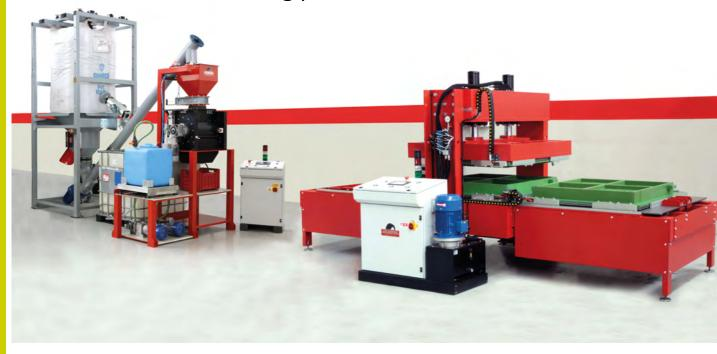
Metamorphisis II transforms recycled rubber granules or frayed rubber into superb shock proof flooring, residential and industrial flooring, flooring for livestock, or self-locking paving. Shapes and pavers are added by different shaped mold.
