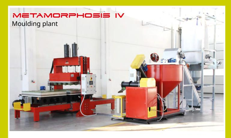
Metamorphisis IV transforms recycled rubber granules or frayed rubber into industrial wheels for trolleys and bins. Customized molds also produce articles for the urban, industrial and civil building industry, animal husbandry, etc.
