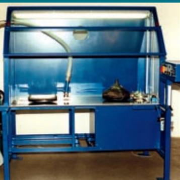
*The manually operated system is a simple version, it can process CRTs ranging from 8" to 40". The operator measures, scratches and applies the hot band manually.*
